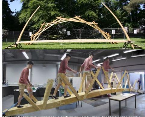
"Jigsaw" bridge with compressive arch plywood box deck, braced by rope handrail
