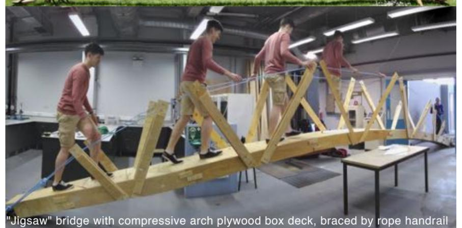
"Jigsaw" bridge with compressive arch plywood box deck, braced by rope handrail
