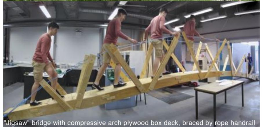
"Jigsaw" bridge with compressive arch plywood box deck, braced by rope handrail
